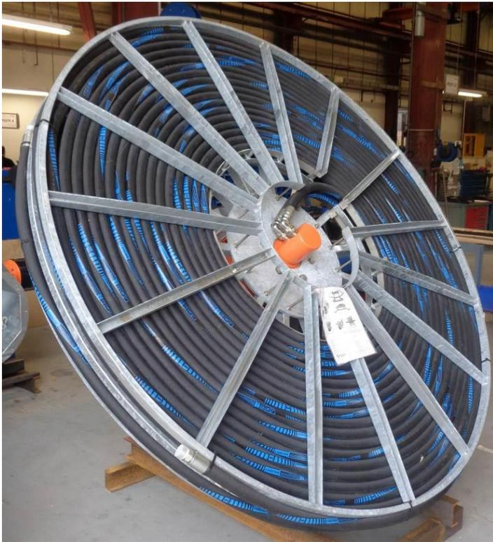
*Caption: Hose reel with rotary transmitter and a 2 x 1" connector for the supply of argon gas with two hoses*
